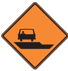
Low shoulder ahead. Difference in elevation due to construction
