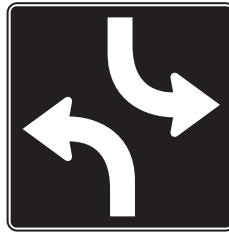
Two-way left-turn lane
