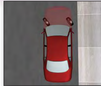
uphill with curb
