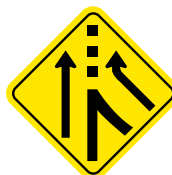
Free flow (added lane)
