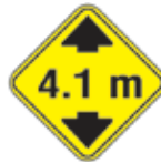
Low structure clearance 4.1 metres
