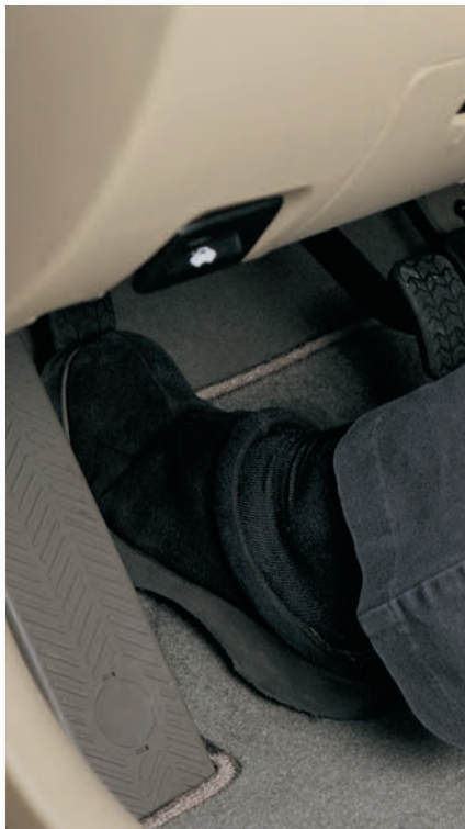
Left foot brace
