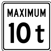
Weight limit of vehicle permitted on highway or bridge expressed in tonnes
